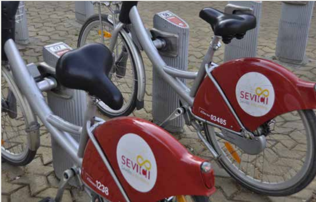
Turning the seat around flags maintenance staff that the bike needs to be serviced.
