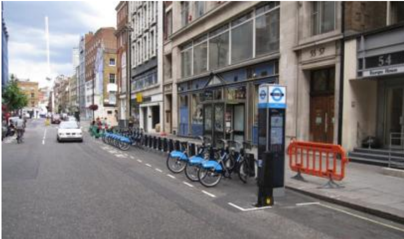
Figure 6. A cycle sharing station can fit in a 2 m wide parking lane.
