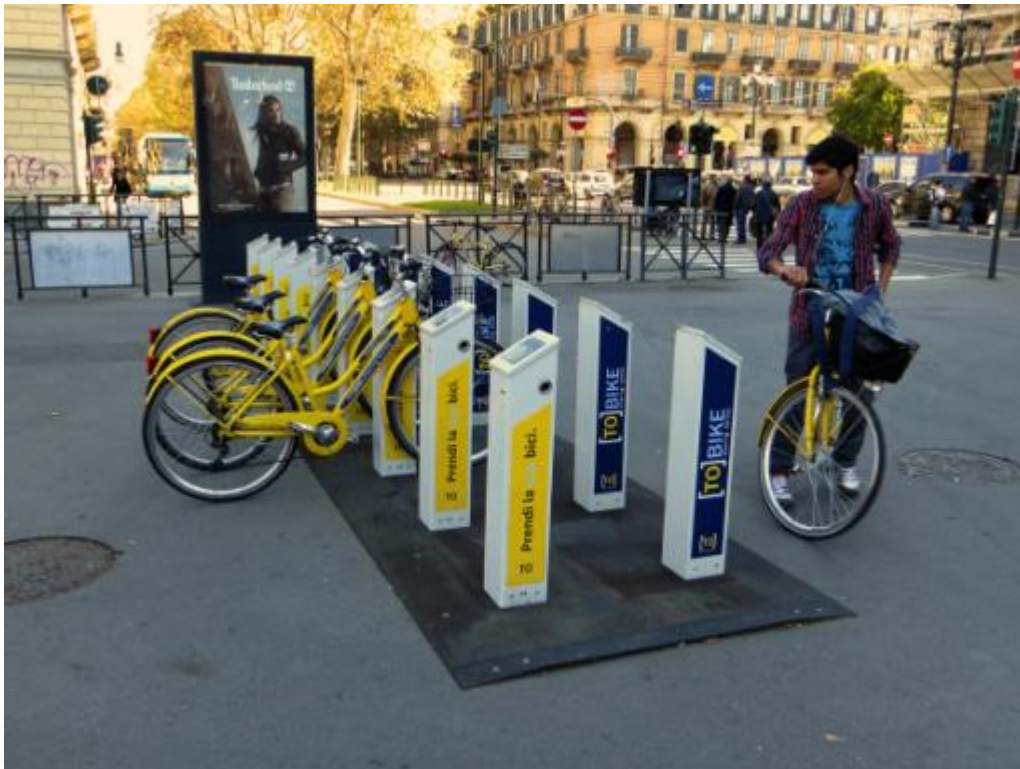
Figure 1. Modern cycle sharing systems feature a dense network of stations. A user checks out a cycle using an RFID-enabled smart card and can return it to any other station.
