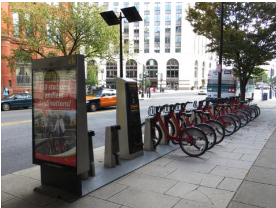
Figure 4. A typical cycle sharing station includes docking positions, a user terminal, and space for advertising.
