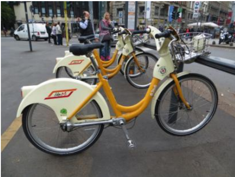
Figure 2. A unique, robust cycle design is critical the branding and reliability of the system. The cycle should be a unisex model with an adjustable seat.
