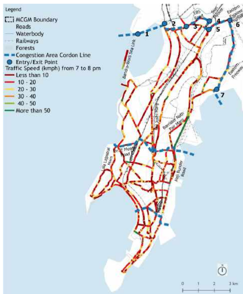
Figure 27 Traffic Speeds in the Island City of Greater Mumbai 64 and potential congestion pricing cordons
