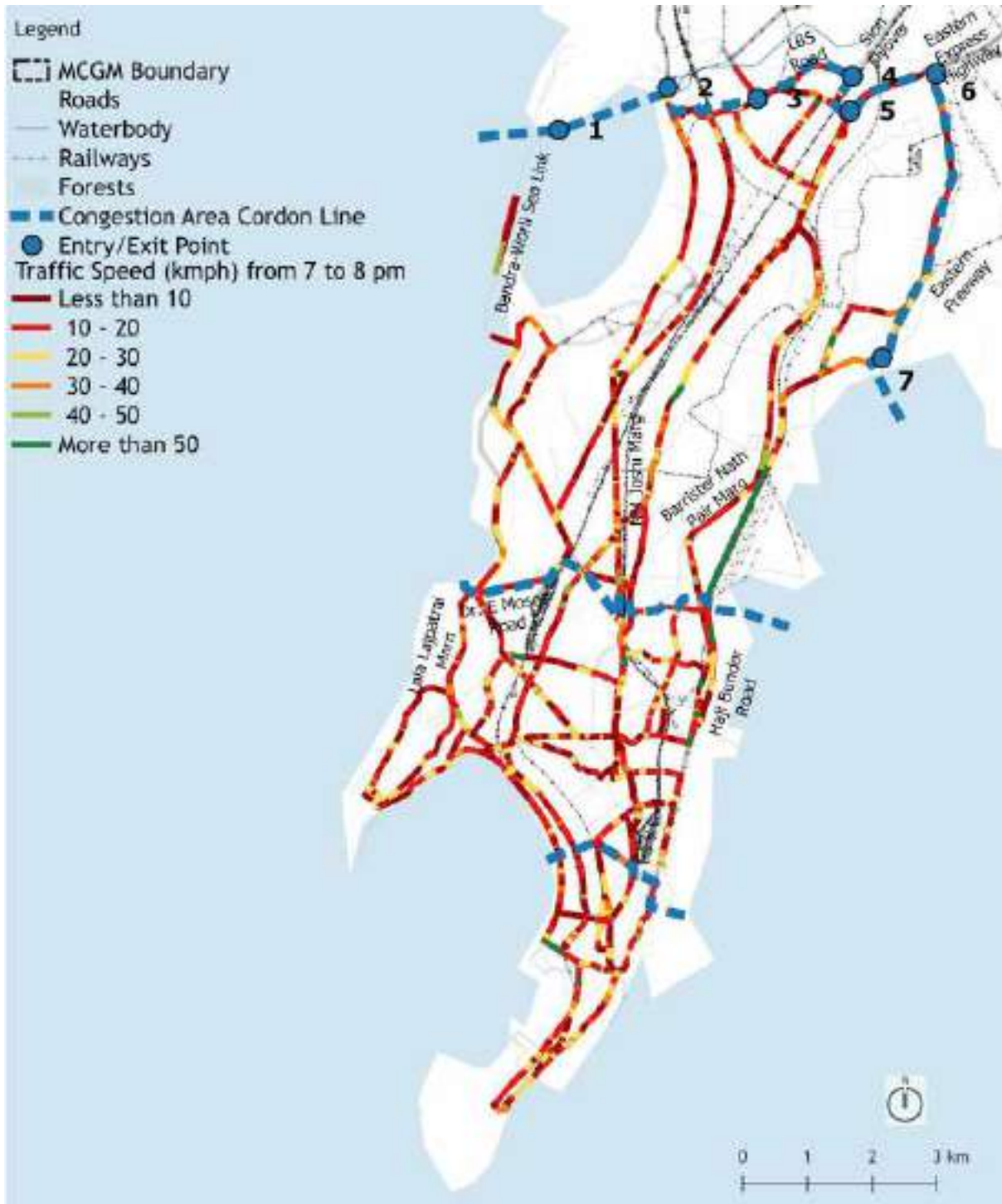
Figure 16 Traffic Speeds in the Island City of Greater Mumbai and potential congestion pricing cordons
